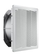
FPF series exhaust filter and filter fans represents a side-mounted cooling solution with filtered ambient air to maintain optimum ventilation inside the electrical cabinets. These units have a flat external profile and a quick snap-on fastening system with elastic hooks. Available in different range of sizes, airflow ratings and configurations.
