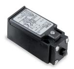
The limit switches ensure safety during maintenance work inside the electrical panels. They are applied on the frame of the cabinet and can turn on the lights, turn off a fan or a heater or cut off the power supply in general when the door is opened or closed.
